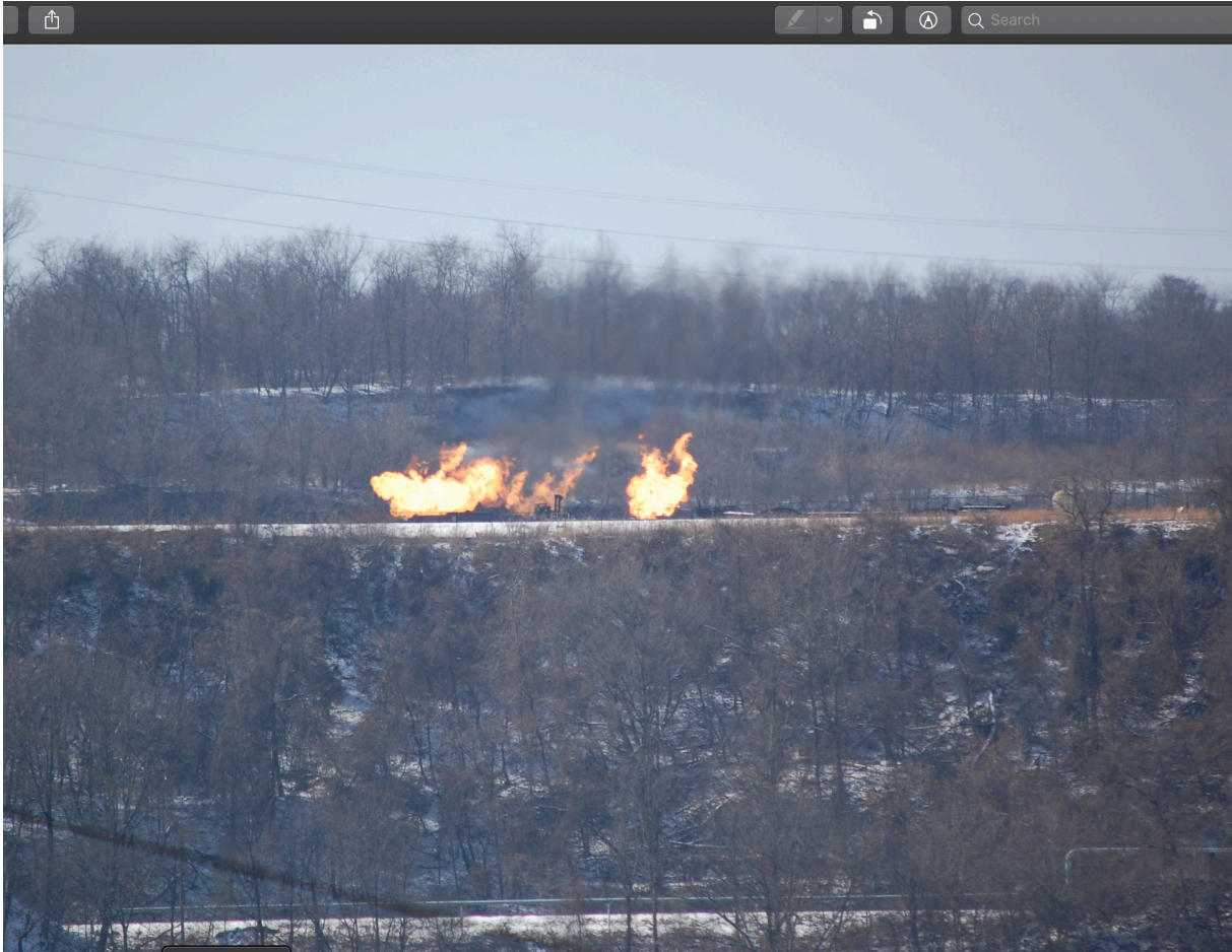
Figure 3: Close up of view of flare of un-desulfurized coking gas from Glassport, PA
